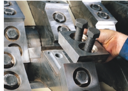
With the special Ecofix system, tooling replacement does not require removal of the rotor shaft - an important availability advantage.
