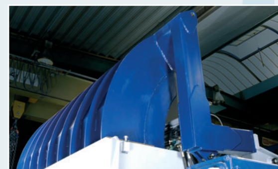
The pusher system prevents of material deadlock
