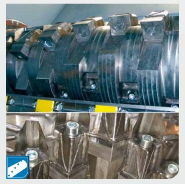
Single Shaft Milling Rotor High shredding quality/-performance at low-vibration run by spiral-shaped knife assembly
