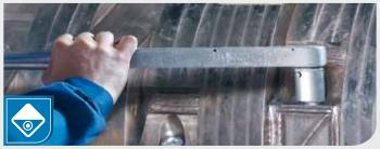
Monofix-System Knife fixation using only one screw. Quick change of knives
