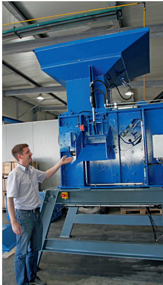
◀ 2 Pilot plant at ATM Recyclingsystems with Andreas Schmid, who basically carried out the research works regarding the briquetability of aluminium swarf
