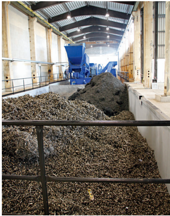
4 ▶ Swarf storage bunker Spänevorratsbunker
