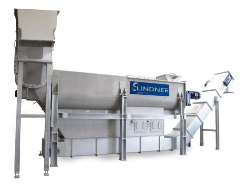
As a washing system for pre-shredded highly contaminated post-consumer plastic waste, the new Rafter takes its place in the recycling line between the Micromat WS wet shredder and a downstream Loop Dryer. All three systems form part of the new washing machine concept for plastics presented by the Austrian Lindner Group. © Lindner washTech
